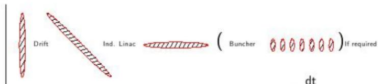
Bunched Beam Rotation with 200 MHz RF (Neuffer)
