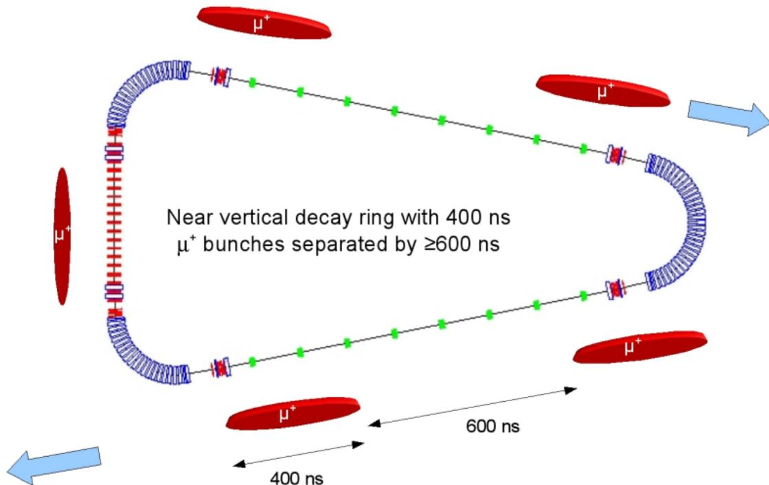
$\sim 300$  m production straights; two detector sites; efficiency  $\sim 48\%$ ;
