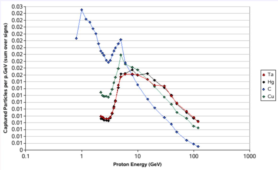
MARS15 output suggests optimum proton beam energy range of 5–15 GeV.
