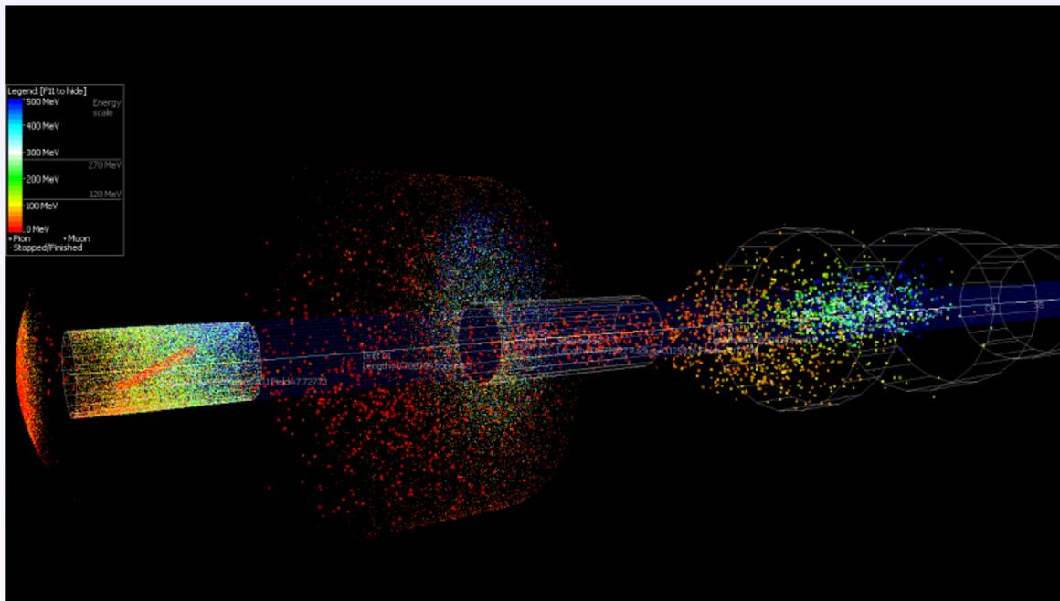
Target is a tilted 20 cm long Ta rod inside a 20 T solenoid
