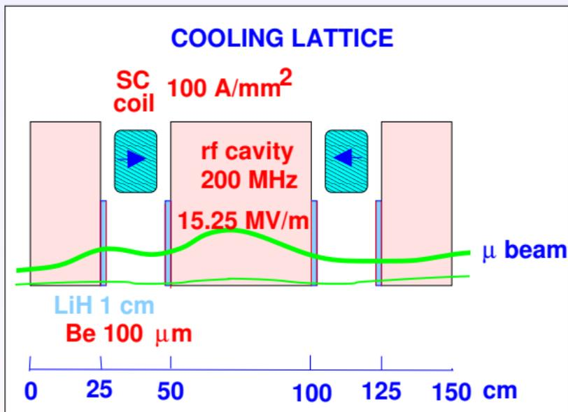
1. Liquid hydrogen absorbers remove momentum in all directions
