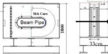
Japan Ferrite Loaded RF (cf PRISM)
