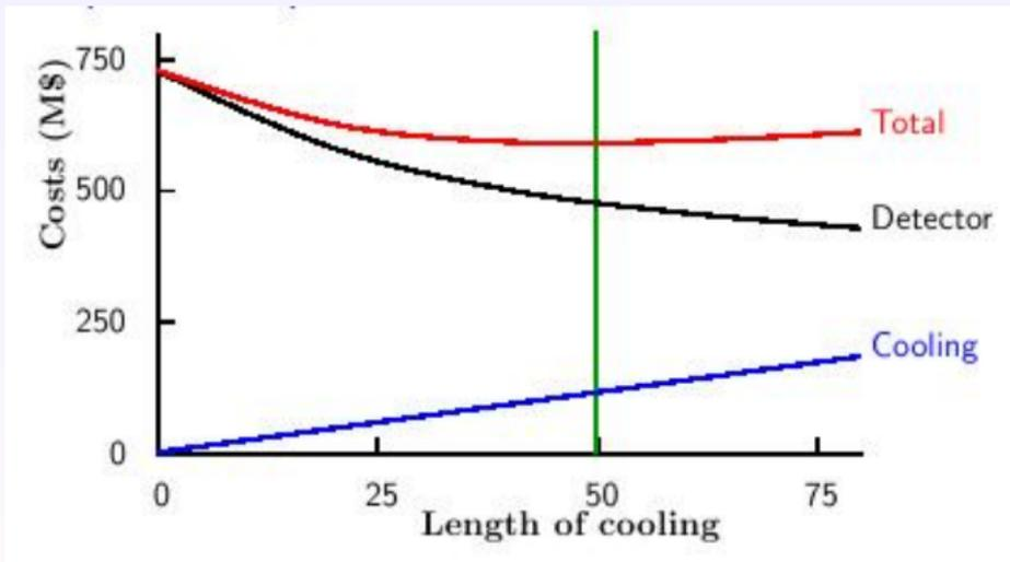
Assuming two detectors, total cost minimum for 50 m of cooling.
