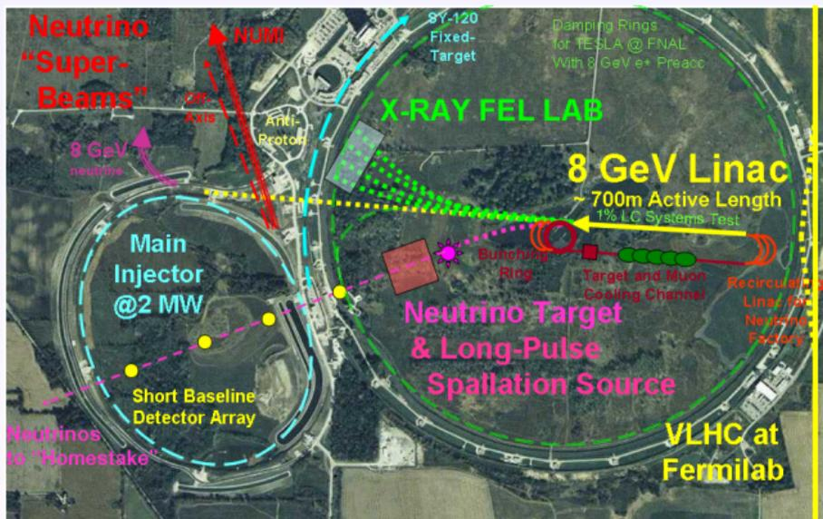
8 GeV Linac can produce streams of  $1.5 \times 10^{14}$  protons at up to 10 Hz
